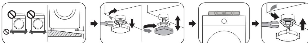
Adjust the levelling feet to level the washing machine. Once the washing machine is level, tighten the locking nuts with a spanner.
