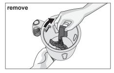
If the coupler is removed (the blade sticks together with the axis), washers will come off when you take blade assembly out of the jar.
