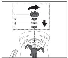
**8.** Check that all parts are properly connected before use.
