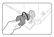
**1.** Put a floor-cloth or towel under the Pump filter. Turn the filter knob anticlockwise to remove.
